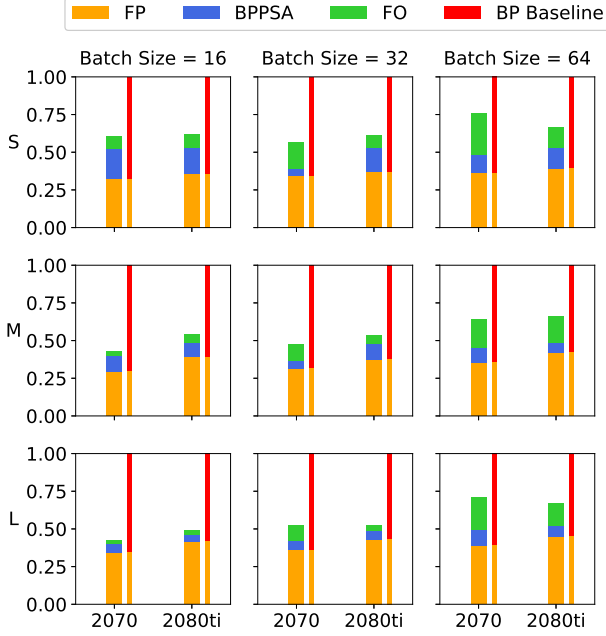
Figure 9: The runtime breakdowns in the GRU end-to-end benchmark as the dataset type ( S , M , L ) and batch sizes B vary. FP represents the forward pass; FO represents the forward pass overhead of computing the transposed Jacobians; BP represents the BP baseline; and BPPSA represents the backward pass via BPPSA. The measurements are normalized by the total runtime of the baseline ( FP + BP ).
